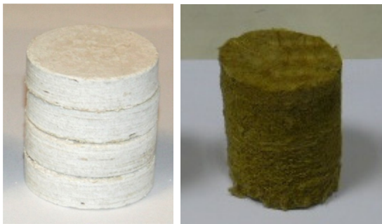
Figure 1 A typical test specimen of the calcium silicate board to the left, and of the mineral wool to the right.
